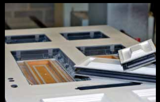
Door after routing operation
